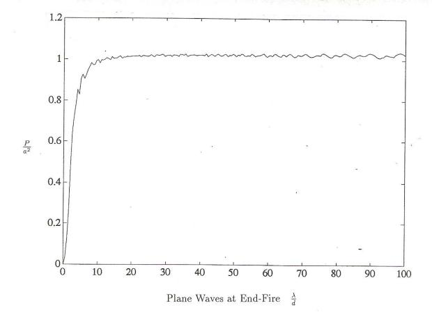
Figure 13: Treatment of singularities with 'exponential' spacing of hydrophones
